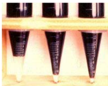
Samples taken at different point across a pipeline profile
